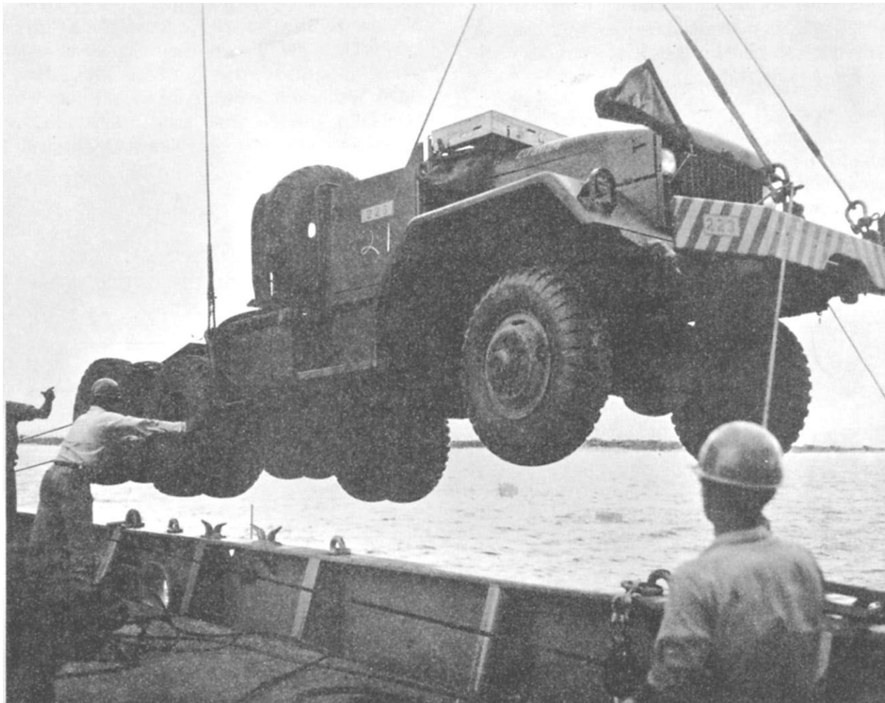
Figure 9-21.—Bridle legs may be attached to hoisting padeyes of unloaded military vehicles.
